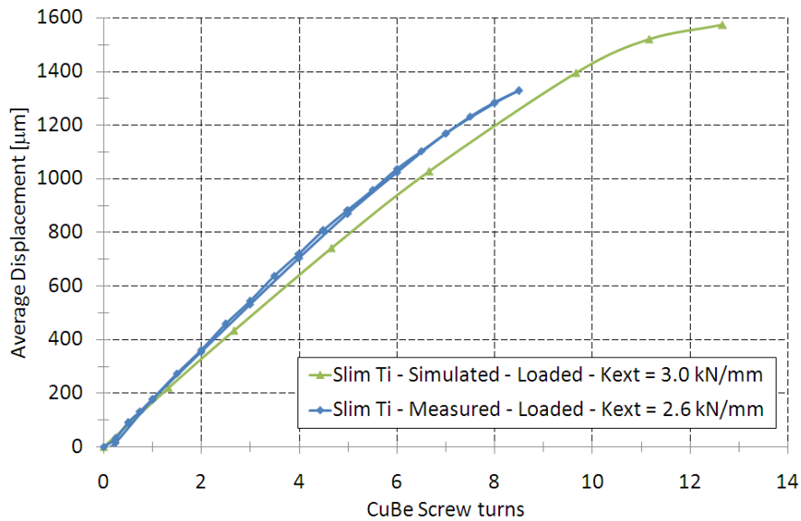
Fig. 6.41 - comparison of experimental and numerical data at the piezo position for the loaded case
