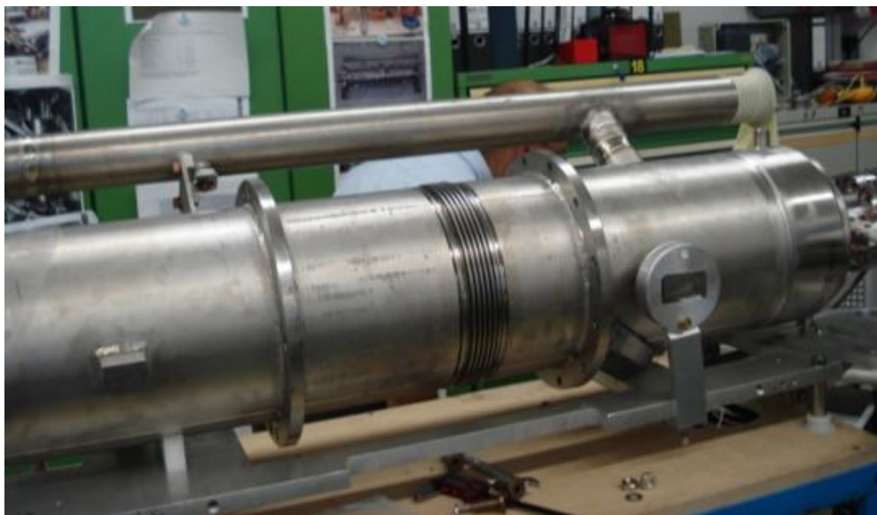
Fig. 6.45 – Z86 and modified He tank with support disks and bellow, ready for Blade tuner installation
