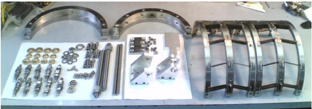
Fig. 6.44 – complete set of Slim_SS tuner elements for the DESY cold test
