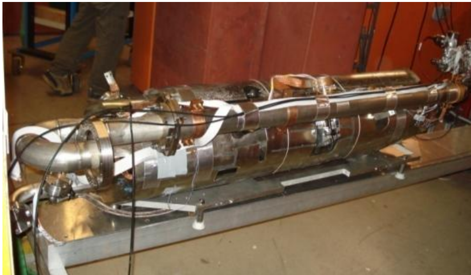
Fig. 6.47 – Z86 right before insertion in CHECHIA, the magnetic shielding is visible around the He tank
