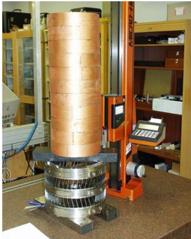
Fig. 6.12 - experimental compression test on Blade Tuner
