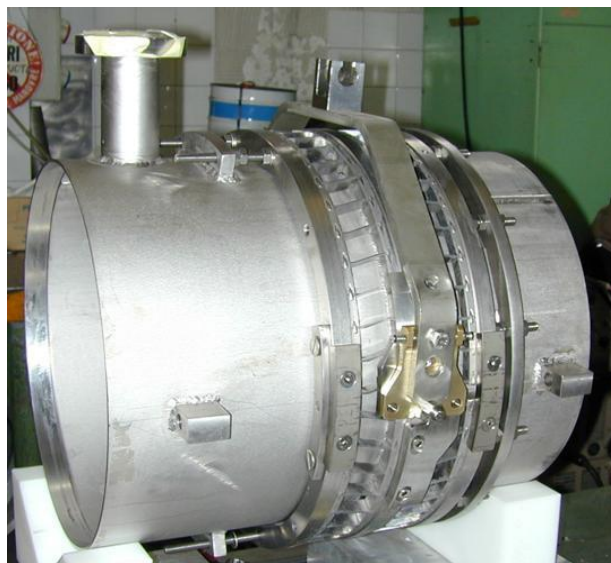
Fig. 6.62 – the coaxial Blade Tuner for the low- \beta proton SC cavity
