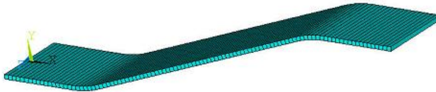
Fig. 6.7 – finite element model of a single blade
