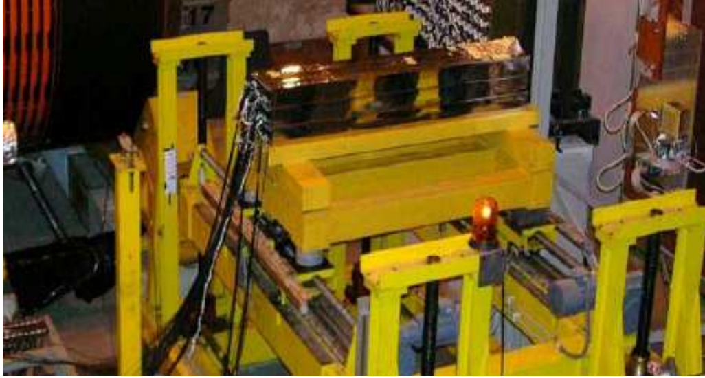
Figure 4: The PSD super-module positioned in the NA61/SHINE experiment downstream of the MTPC hut.
