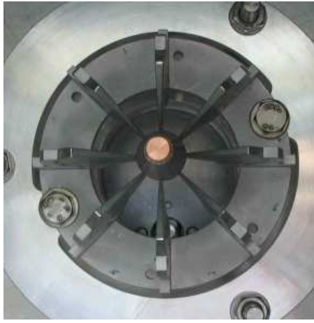
Figure 4: Magnetic Mini-Orange filter and transport system, consisting of eight wedge-shaped permanent magnets arranged around a central Pb absorber.
