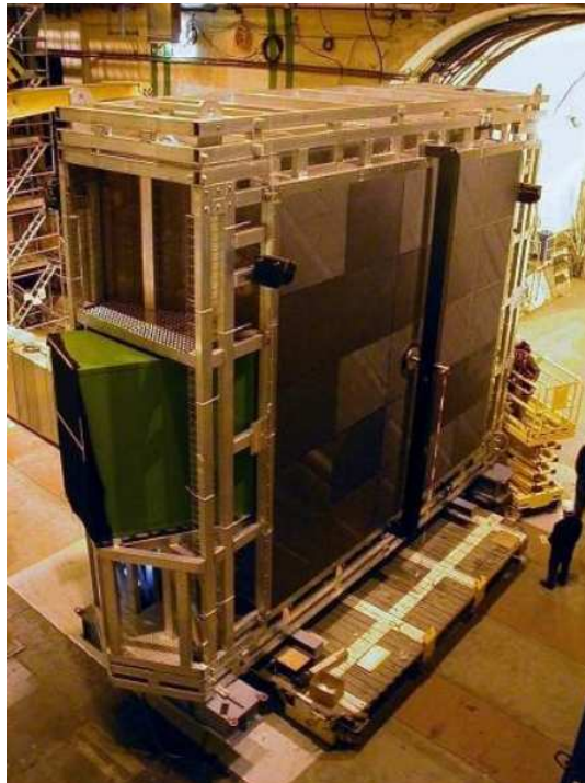
Figure 3.7: The LHCb RICH2 detector during installation at IP8 [50]. The green box on the left of the photograph is the magnetic shield which contains the photodetectors.
