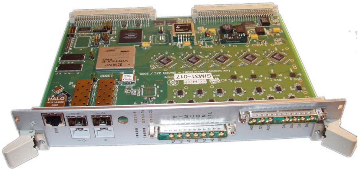
Figure 6.4. New control board.
