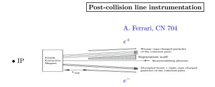
Lots of observables:  $e^-, e^+, \gamma$  energies, sizes, polarization, etc. Challenges: design, losses, beam sizes  $\approx 40$  cm,  $\Delta E/E_0 \approx 50\%$ , etc.  $\rightarrow$  A lot to do!
