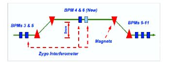
4 Bends chicane: The energy is inferred from BPMs. Drawback for CLIC: too long!, alternatives:  $\rightarrow$  Compton backscattering (under study @ ILC)  $\rightarrow$  using a single bend?
