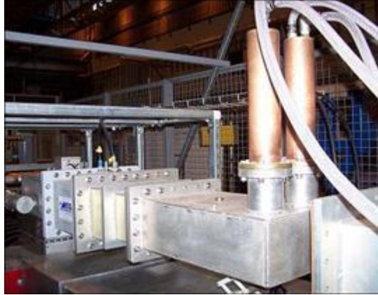
Fig. 9: Klystron output with bi-directional coupler and RF load
