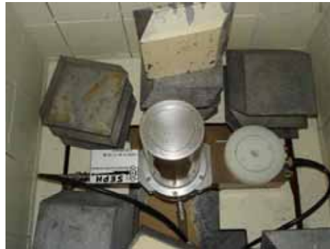
Figure 43: The detector with its Pb shielding
