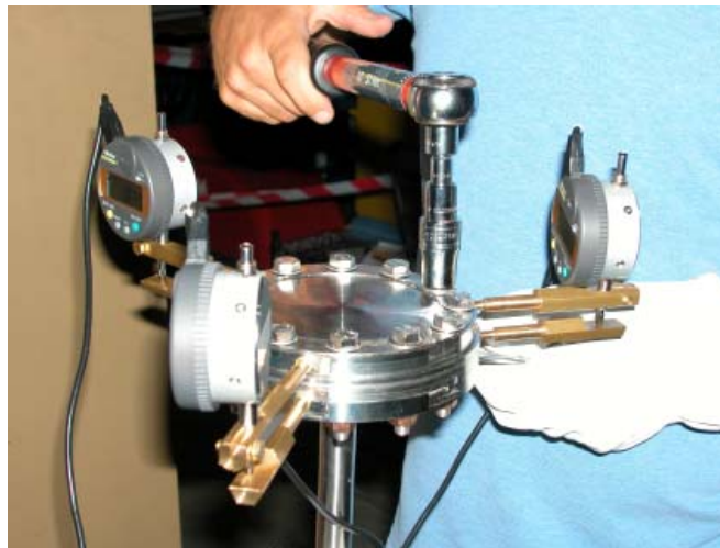
Figure 22 : manually compression test using a torque meter on the bolts head: the leak detector is connected to the bottom flange.
