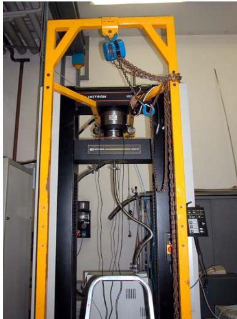
Figure 5: the Instron machine used for the compression tests.
