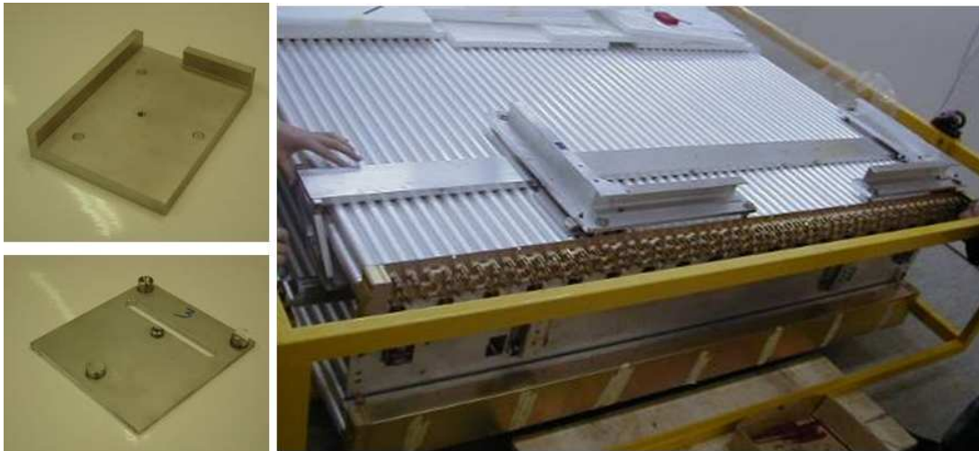
Fig. 15: Support platform for the praxial sensors (top left) and for the projective and BIR-BIM sensors (bottom left). The photo on the right side shows the positioning of two platforms (projective and BIR-BIM) by using L shape template frames. The position along the tube direction refers to the praxial platform mounted on the inner face of the multilayer by means of a calibrated ruler.
