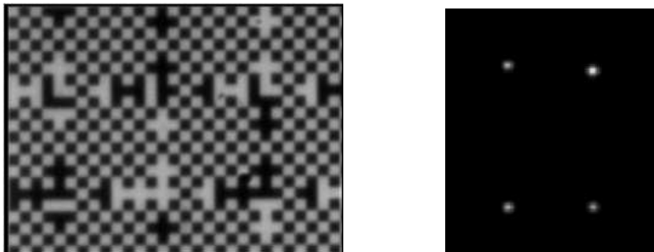
Fig. 4: Left: RASNIK chess board pattern seen by the CMOS. Right: Image of LED spots seen by a SaCam.
