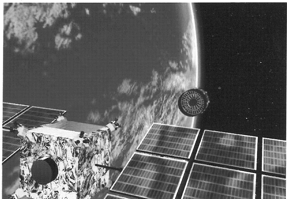
Figure 9. XEUS in its operational configuration. The DSC (foreground) maintains its position at the focus of the MSC mirrors some 50 m away to within \pm 1 mm
