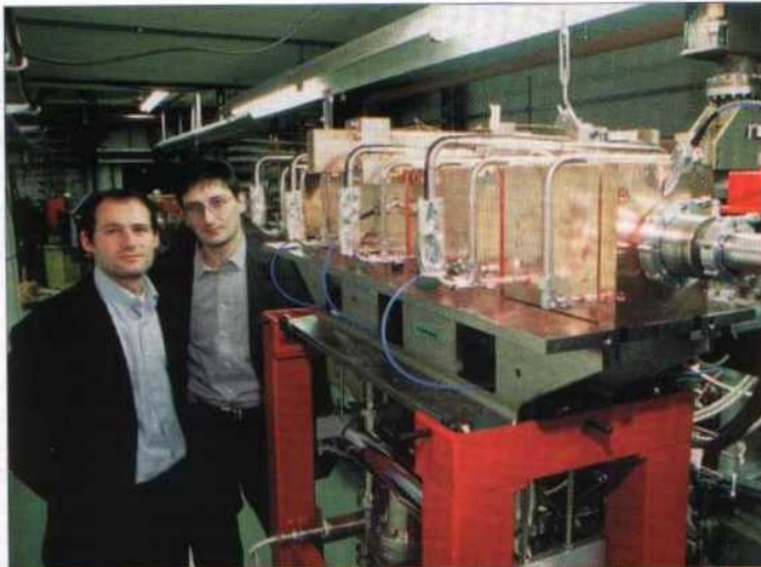
Riccardo Zennaro and Paolo Berra of the LIBO Linac Booster collaboration with the first LIBO module installed and awaiting power tests at CERN.
