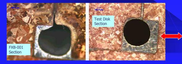
The brazing technique is fundamental for a good joint and it is connected to: RF contact, vacuum tightness, thermal conductivity
