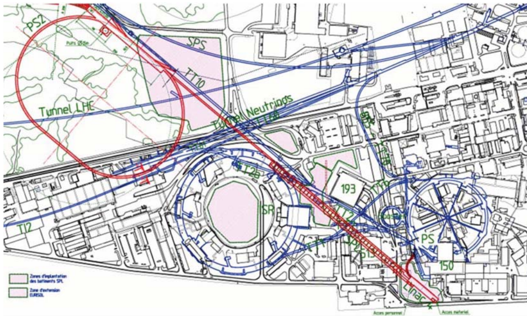
Figure 1: Layout of the new proton injector complex at CERN.
