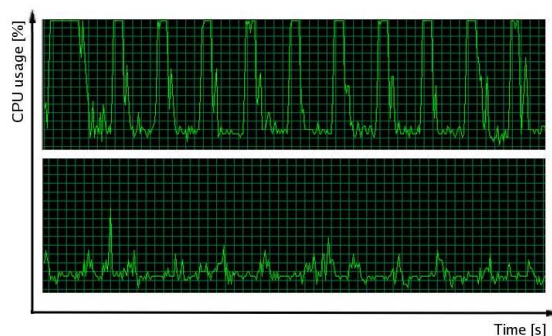
Figure 18. CPU consumption of the MoPS project PC during barrel cosmics run. The plot shows regular peaks at 100% with a period corresponding to the MoPS reading rate (15 seconds) for both PVSS application and OPC server (top) and for the OPC server in stand alone mode (bottom).
