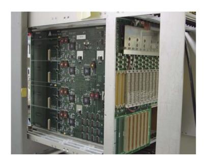
In order to check possible transmission errors, a checksum is generated in the Input Cards on each fragment, transferred to the Builder Card, and compared with a checksum being generated.
