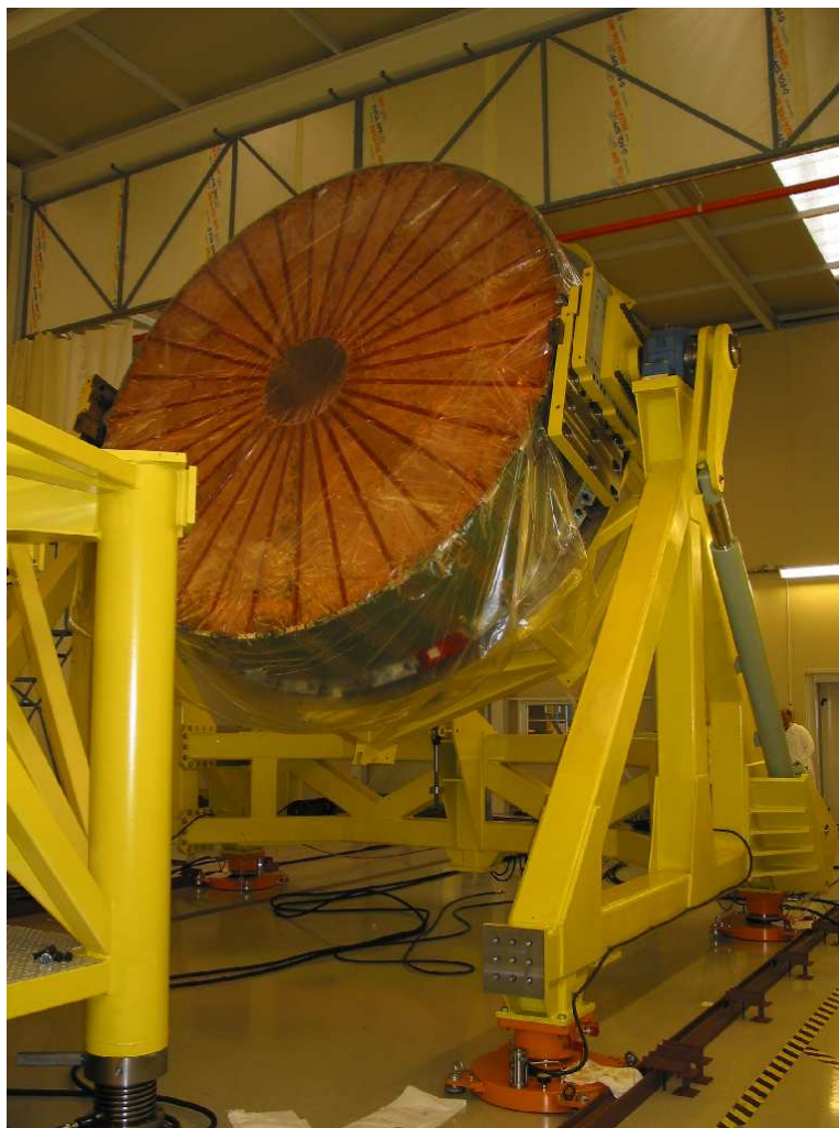
Figure 13. One of the two HEC1 wheels being rotated to the vertical orientation with the custom designed tooling after having been moved from the wheel assembly area. The wheel assembly stand can be seen on the left.
