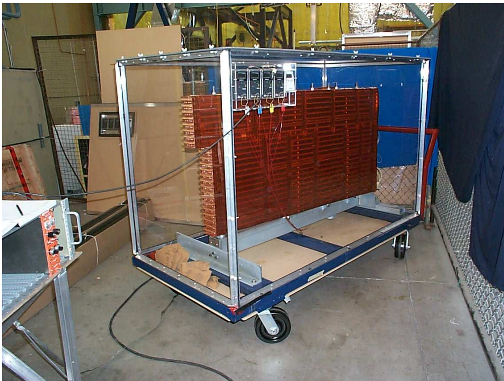
Figure 9. Module undergoing a long term HV test at 1800 V for 10 days. The module is bolted on its shipping frame, and stored in a clean area or box. The relative humidity is monitored as well as the currents in the liquid argon subgaps.
