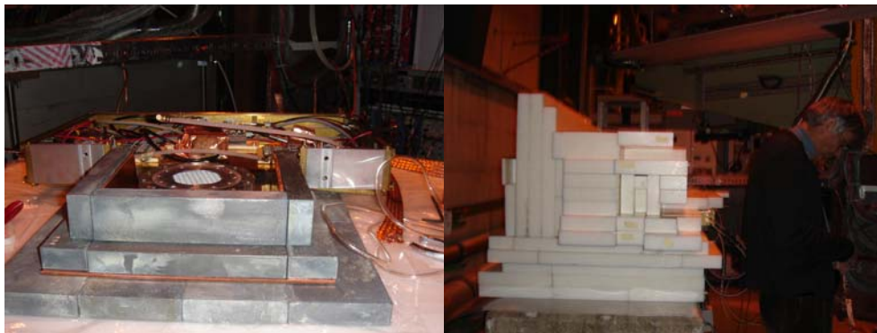
Figure 15: On the left, the Micromegas detector dismounted of the CAST magnet lying on a concrete block and partially covered by copper and lead. On the right, final set-up of the shielding test with Micromegas detector completely covered by copper, lead, polyethylene (white blocks).
