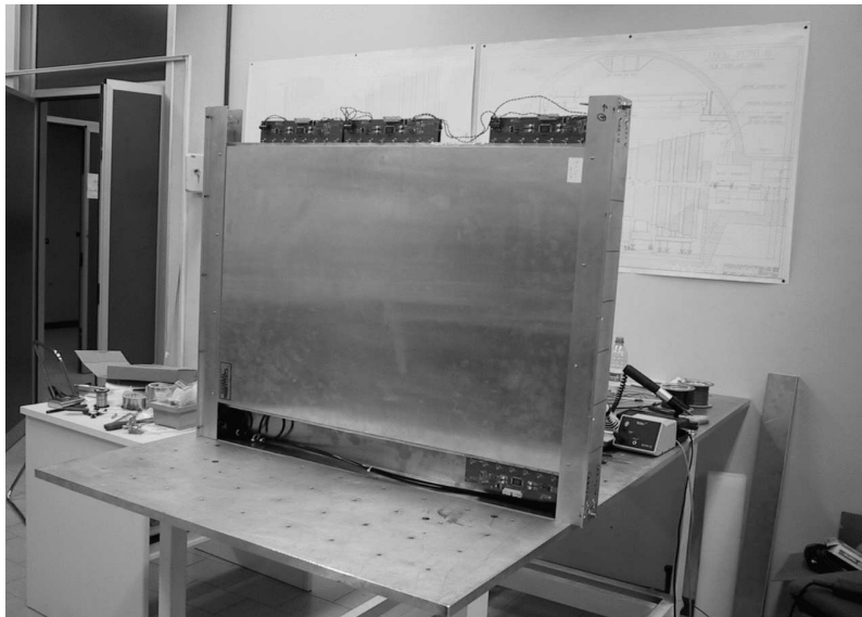
Figure 2.5: RPC detector during the assembling. The front-end boards are visible.
