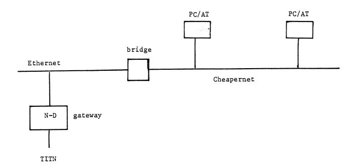
The main disadvantages of Ethernet are its price and difficult connectivity which is illustrated above. It permits relatively short distance (~ 700 m without repeaters) which may not be a drawback for a LAN limited to the main control room.
