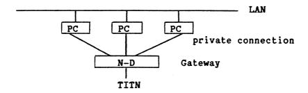
The first scheme is more elegant but as opposed to the second one it merges on the LAN the control traffic with the N-D gateway and the development traffic between the PC's. The main difficulty with the second scheme is that the private connection which can be used are limited in bandwidth.
