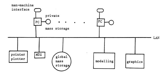
The important point to underline about this diagram is its open architecture. If we choose the network and engineer the software properly, it will be possible, and may be easy, to introduce new ideas or products in the future and in addition, it offers the possibility of a progressive implementation.
