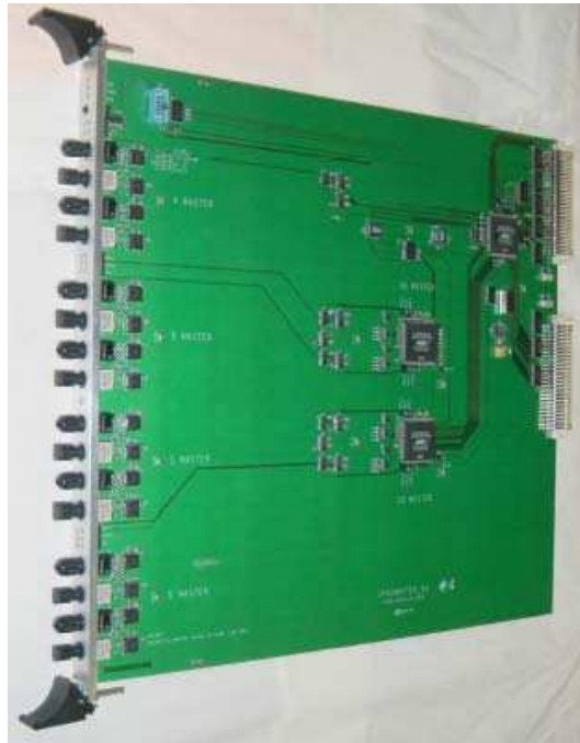
Figure 13. Photograph of a SPAC Master board equipped with 4 SPAC links.
