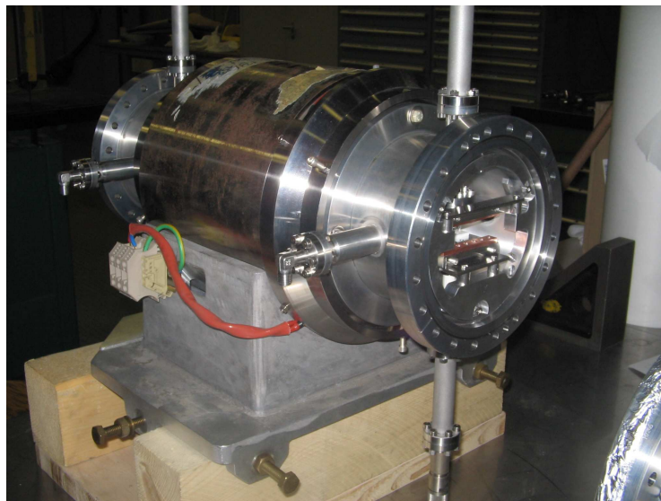
Figure 2.16: The chopper structure inside the quadrupole (top) and a detail of the deflecting plates
