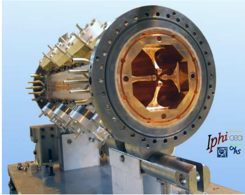
Figure 2.5: Module 1 of the IPHI RFQ after brazing
