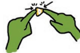
If you have more than one LED connected in parallel, and only some of them are on, the most likely issue is a weak connection on the LEDs that aren't turning on. You can fix these weak connections by taping conductive fabric patches between the LED's metal pads and the underlying copper tape.
