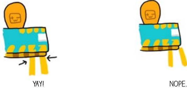
**7. Is the copper tape really bumpy or wrinkly?** If so, sometimes bumps and wrinkles can prevent solid connections to your LEDs or Chibi Chip. If this is the case, try smoothing out the tape by rolling over it with the flat side of a pen or pencil.
