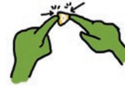
MAKE A STRONG CONNECTION! TRY PRESSING HARD ON THE METAL PADS OF THE LED.
