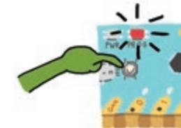
DID THE PROG LIGHT TURN STEADY RED BEFORE PROGRAMMING? IF NOT PRESS AND HOLD THE PROG BUTTON UNTIL IT TURNS RED AND TRY UPLOADING AGAIN.
