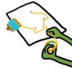
2. Lay copper tape going from GND to each of these dots.
