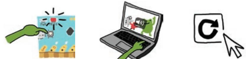
DID THE PROG LIGHT TURN STEADY RED BEFORE PROGRAMMING? IF NOT, PRESS AND HOLD THE PROG BUTTON UNTIL IT TURNS RED AND TRY UPLOADING AGAIN.
