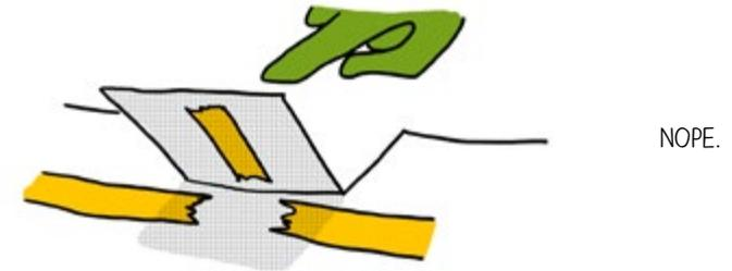
**Make the copper tape patch large and the circuit gap small.** This makes it easier for your switch to close the circuit. This is especially important for more advanced switches, such as the wind sensing switch (page 3-28), where the switch isn't actually pressed by hand.
