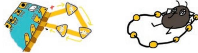
Since the LEDs are in a line, the required voltage also adds up so we'll need a higher voltage power source. For example, since each LED sticker requires 2.5V to shine brightly, to turn on 3 LEDs in series we will want a 7.5V power supply. They may still glow with less voltage, but not as bright.
