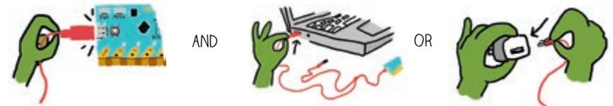
4. Plug the audio end of the programming and power cable into the audio jack of your programming device.
