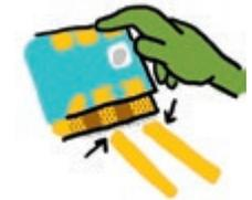
CHECK YOUR ALIGNMENT! MAKE SURE THE GOLDEN METALLIC STRIPES ON THE CHIBI CHIP ARE LINED UP AND MAKING SOLID CONTACT WITH THE COPPER TAPE.
