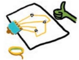
3. Tape copper traces from the programmable pins to the dots, and add your LED stickers!
