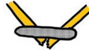
**10. Is your circuit connected at turns and corners?** Copper tape often tears at turns, and it is not enough to stick two pieces of copper tape on top of each other. When making a corner using two pieces of copper tape, reinforce the connection using a conductive fabric patch after sticking down the second piece of copper tape.
