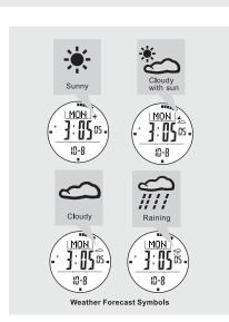
The NOMAD G3-PRO features weather tracking and forecasting icons using changes to the current and past air pressure trends. The symbols are only shown in the current and dual time modes.
