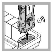
**6.** Wait for the sound alert and/or the meter removal animation (within 1 to 2 seconds), then immediately remove the meter from the sample cup.
