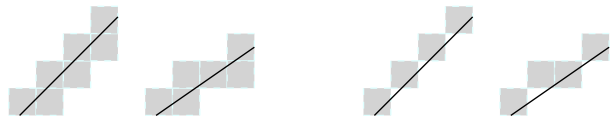
Figure 3.2: Left: Two cases with consecutive grid points where 3 adjacent grid cells are intersected. Right: Iteratively removing intersected grid cells so that no grid point is adjacent to more than 2.
