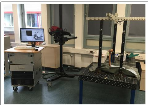
**Fig. 2** Optical 3D scanning setup at AGP Fraunhofer Institute in Rostock. The bone is located on the bench, scanning is performed by the optical scanner on the movable stand and controlled by the computer
