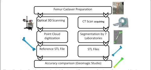
**Fig. 1** Flowchart of methodology. On the left column different steps of making reference model is shown including optical 3D scanning, point cloud digitization and creating STL files. Right column shows that the only CT scan image taken in the study was segmented by 7 laboratories to create 7 STL files
