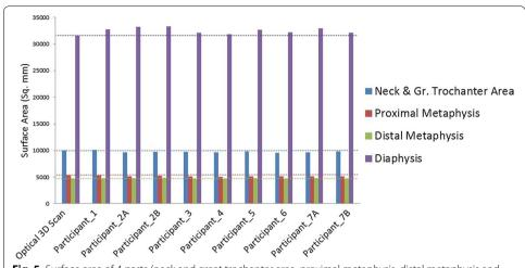
**Fig. 5** Surface area of 4 parts (neck and great trochanter area, proximal metaphysis, distal metaphysis and diaphysis) of the femur obtained from optical 3D scan (reference STL file) as well as 7 participant laboratories
