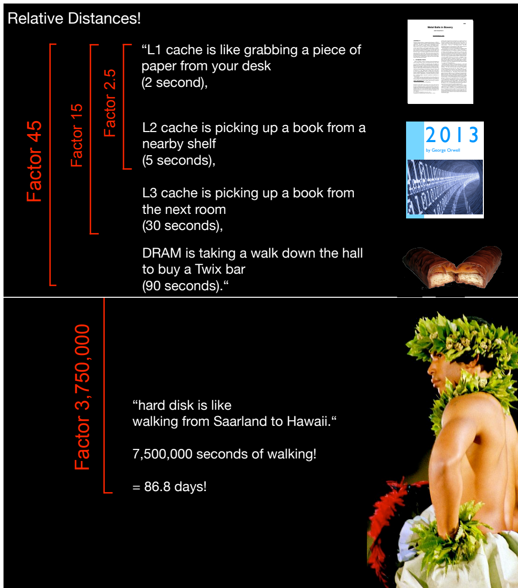
Figure 1.2: Access times translated to a real-life scenario: picking up something from your desk vs walking to Hawaii
