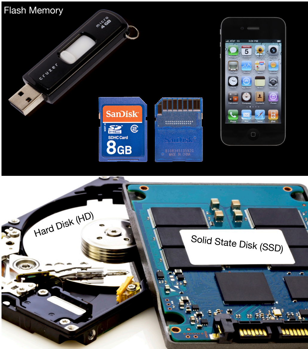
Figure 1.14: Flash memory comes in different form factors, when it comes in the shape of a hard disk we call it solid state disk (SSD).
