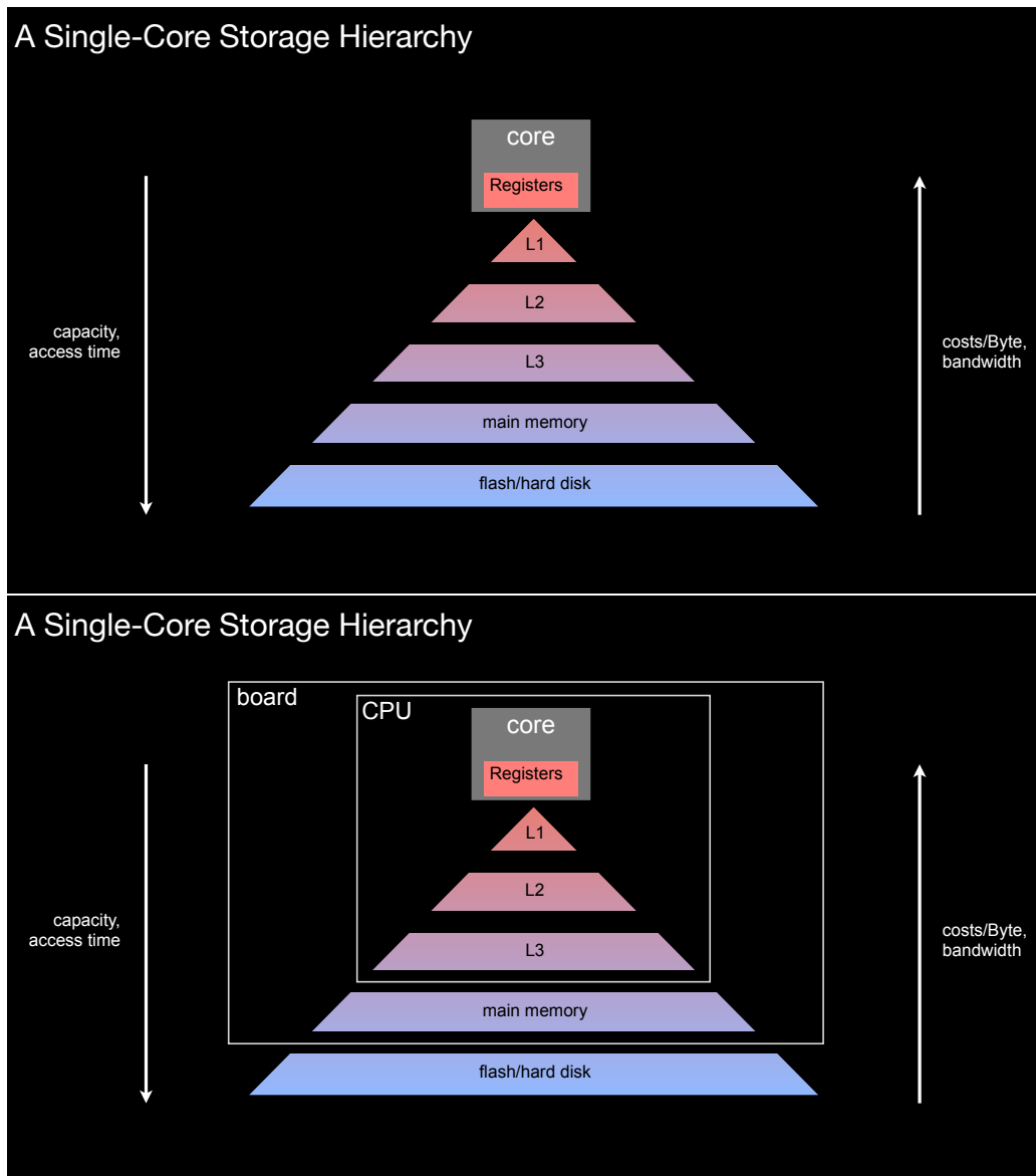
Figure 1.4: A single-core storage hierarchy and how it is mapped to a CPU and the board
