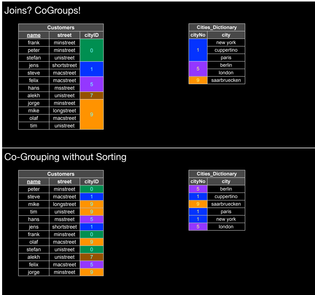
Figure 4.5: Foreign-key constraint typically imply duplicates in one table only; relationship of joins to cogrouping
