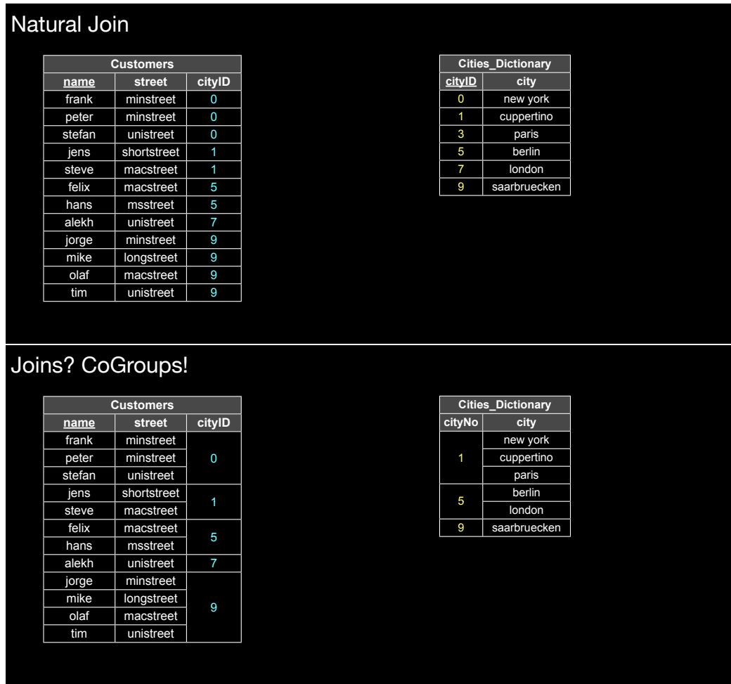
Figure 4.4: Foreign-key constraint typically imply duplicates in one table only; relationship of joins to cogrouping
