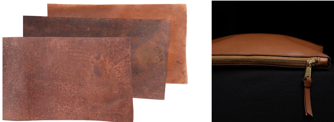
Figure 13. Synthetic leather produced from plant-based oils, and a purse made from this leather (from Natural Fiber Welding, Inc.).
