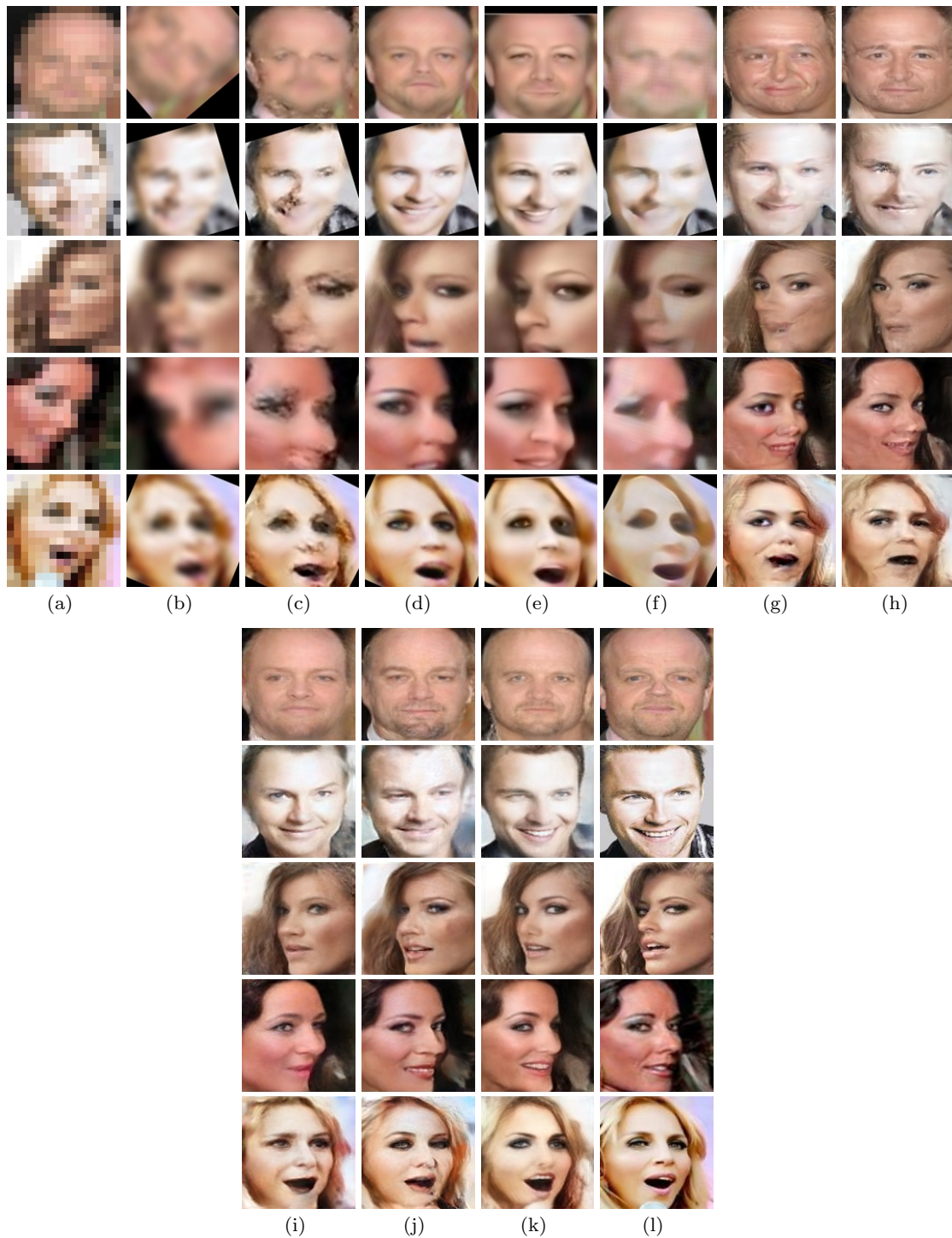
Fig. 9 Comparisons with the state-of-the-art methods on the input images of size 16 \times 16 pixels. The results are obtained in the scenario of first upsampling LR faces and then aligning the super-resolved faces by Bulat et al. 's method (Bulat and Tzimiropoulos, 2017). (a) Unaligned LR inputs. (b) Bicubic interpolation. (c) Kim et al. 's method (Kim et al, 2016a) (VDSR). (d) Ledig et al. 's method (Ledig et al, 2016) (SRGAN). (e) Zhu et al. 's method (Zhu et al, 2016a) (CBN). (f) Chen et al. 's method (Chen et al, 2018) (FSRNet). (g) Yu and Porikli's method (Yu and Porikli, 2017a) (TDN). (h) Yu and Porikli's method (Yu and Porikli, 2017b) (TDAE). (i) Yu et al. 's method (Yu et al, 2018b). (j) Yu et al. 's method (Yu et al, 2018a). (k) Our method (MTDN). (l) Original HR images.
