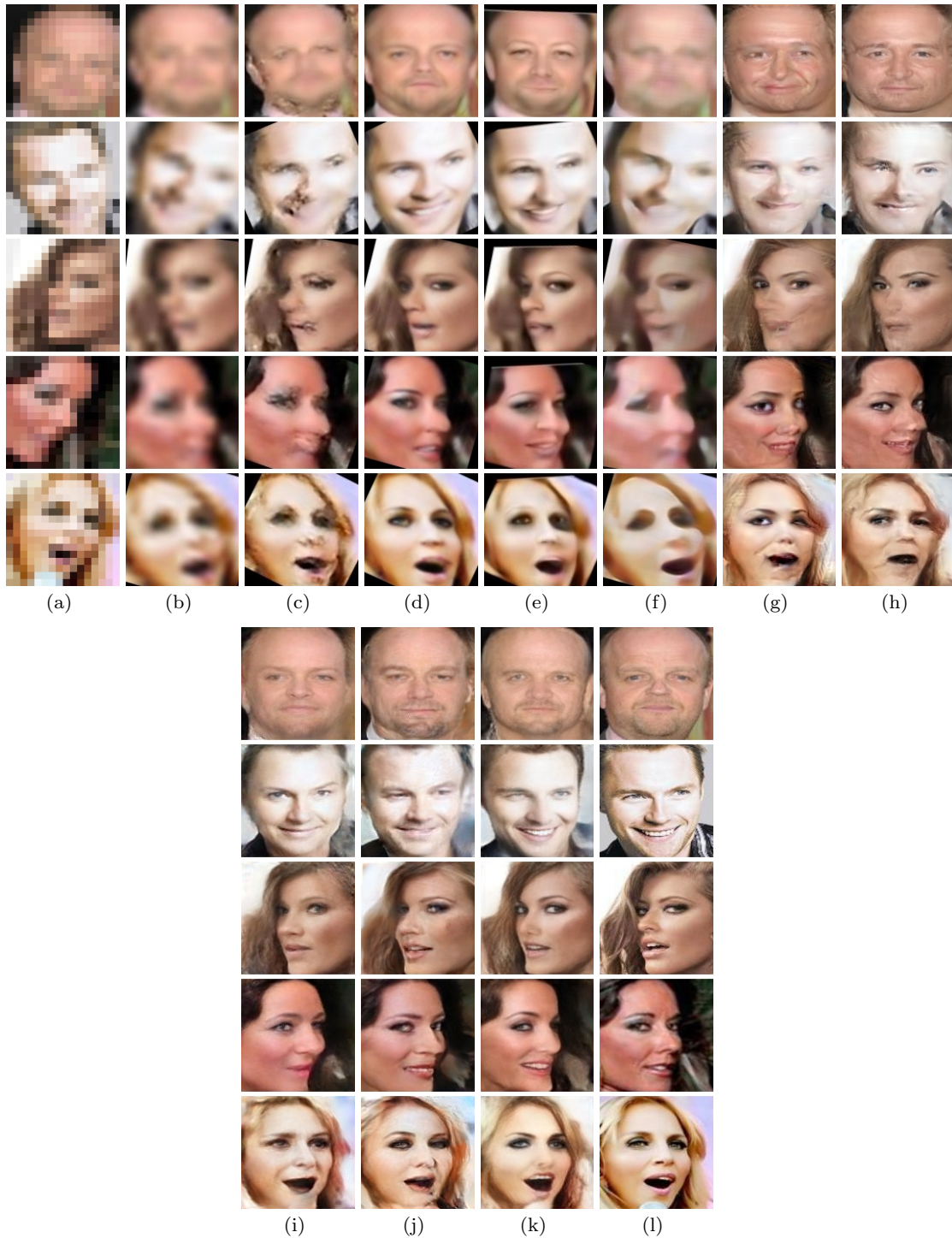
Fig. 8 Comparisons with the state-of-the-art methods on the input images of size 16 \times 16 pixels. The results are obtained in the scenario of first upsampling LR faces and then aligning the super-resolved faces by STN_{HR} . (a) Unaligned LR inputs. (b) Bicubic interpolation. (c) Kim et al. 's method (Kim et al, 2016a) (VDSR). (d) Ledig et al. 's method (Ledig et al, 2016) (SRGAN). (e) Zhu et al. 's method (Zhu et al, 2016a) (CBN). (f) Chen et al. 's method (Chen et al, 2018) (FSRNet). (g) Yu and Porikli's method (Yu and Porikli, 2017a) (TDN). (h) Yu and Porikli's method (Yu and Porikli, 2017b) (TDAE). (i) Yu et al. 's method (Yu et al, 2018b). (j) Yu et al. 's method (Yu et al, 2018a). (k) Our method (MTDN). (l) Original HR images.
