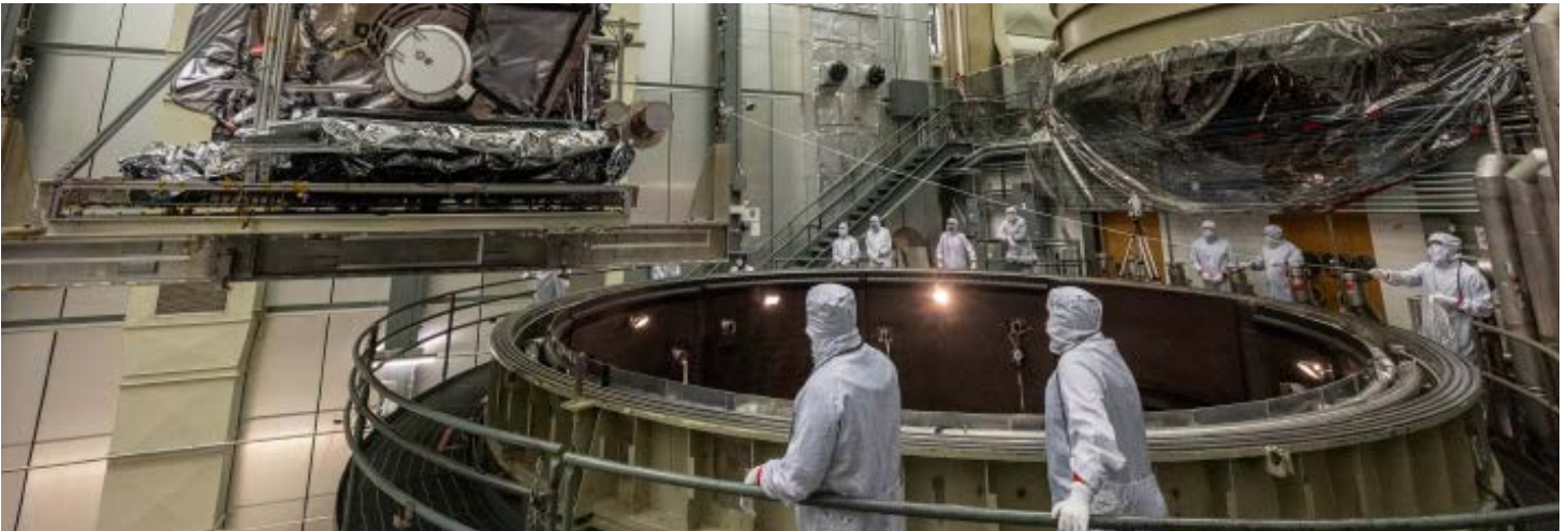
Lockheed Martin thermal vacuum chamber in Littleton, CO (public domain)
