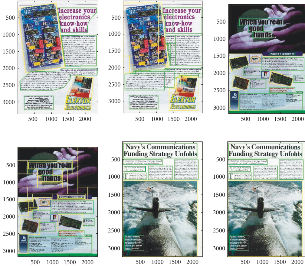
FIGURE 4: Results of manual region detection and automatic polygon partitioning into rectangles. Yellow, green, and blue rectangles and polygons enclose image, text, and graphics regions, respectively.
