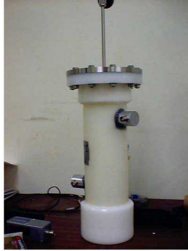
Figure 1. A large-volume droplet detector module (1-litre volume) equipped with piezoelectric sensors glued on the surface for signal detection. The container can be pressurized up to 10 bars. Typical C_xF_y gas loading presently achieved for this type of detector is in the 5-10 g/litre range.
