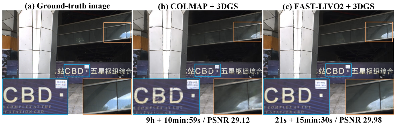
Fig. 16: Comparison of ground-truth image, COLMAP+3DGS, and FAST-LIVO2+3DGS in terms of render details, computational time (time for generating point clouds and estimating poses + training time), and PSNR for a random frame in “CBD Building 01” (see more details on YouTube: youtu.be/aSAwVqR22mo ).
