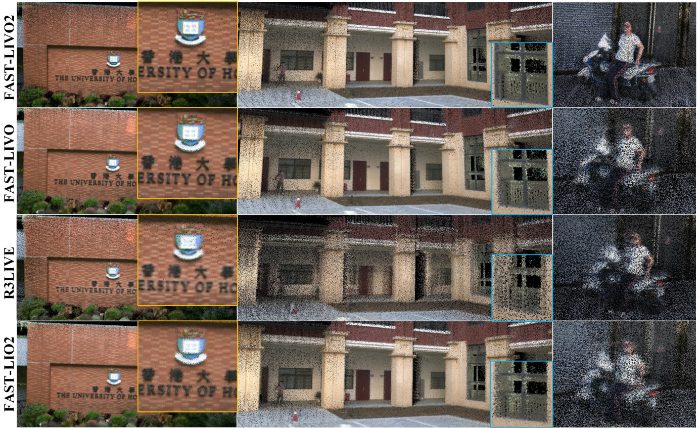
Fig. S9: The real-time mapping results generated online in rich texture and structured scenes. The point clouds from left to right correspond to “HKU Landmark”, “SYSU 01” and “CBD Building 01”, respectively, showing the comparison of colored point cloud accuracy among FAST-LIVO2, FAST-LIVO, R3LIVE, and FAST-LIO2.
