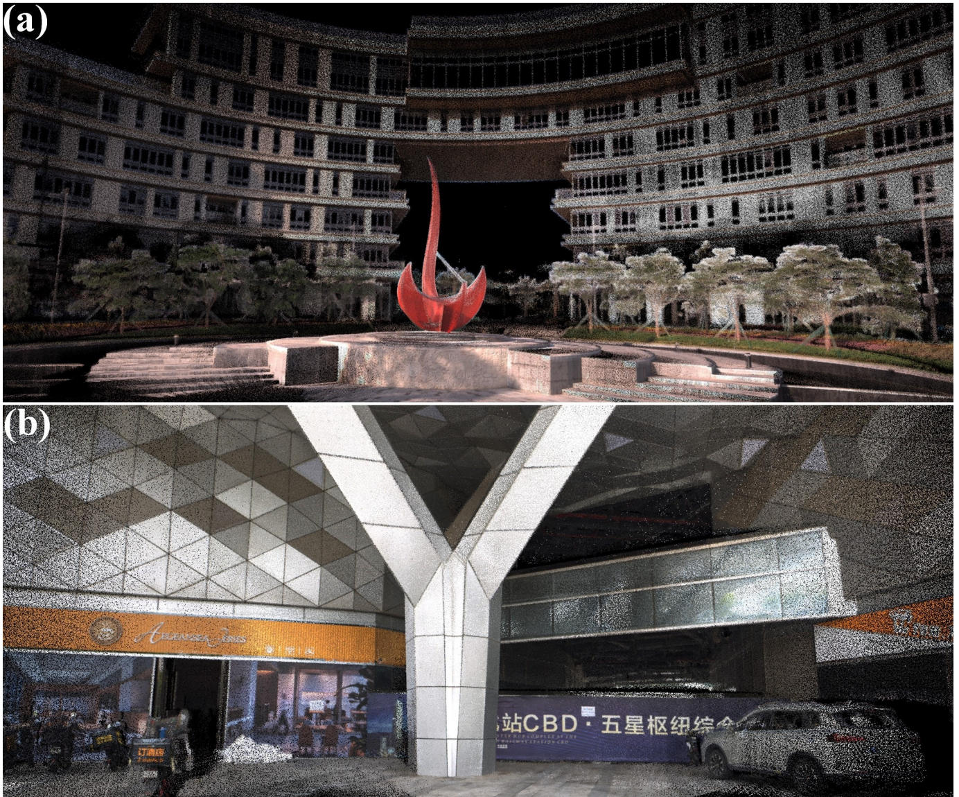
Fig. S13: The real-time mapping results of FAST-LIVO2 in rich texture and structured scenes. (a) “HKUST Red Sculpture”, (b) “CBD Building 01”.
