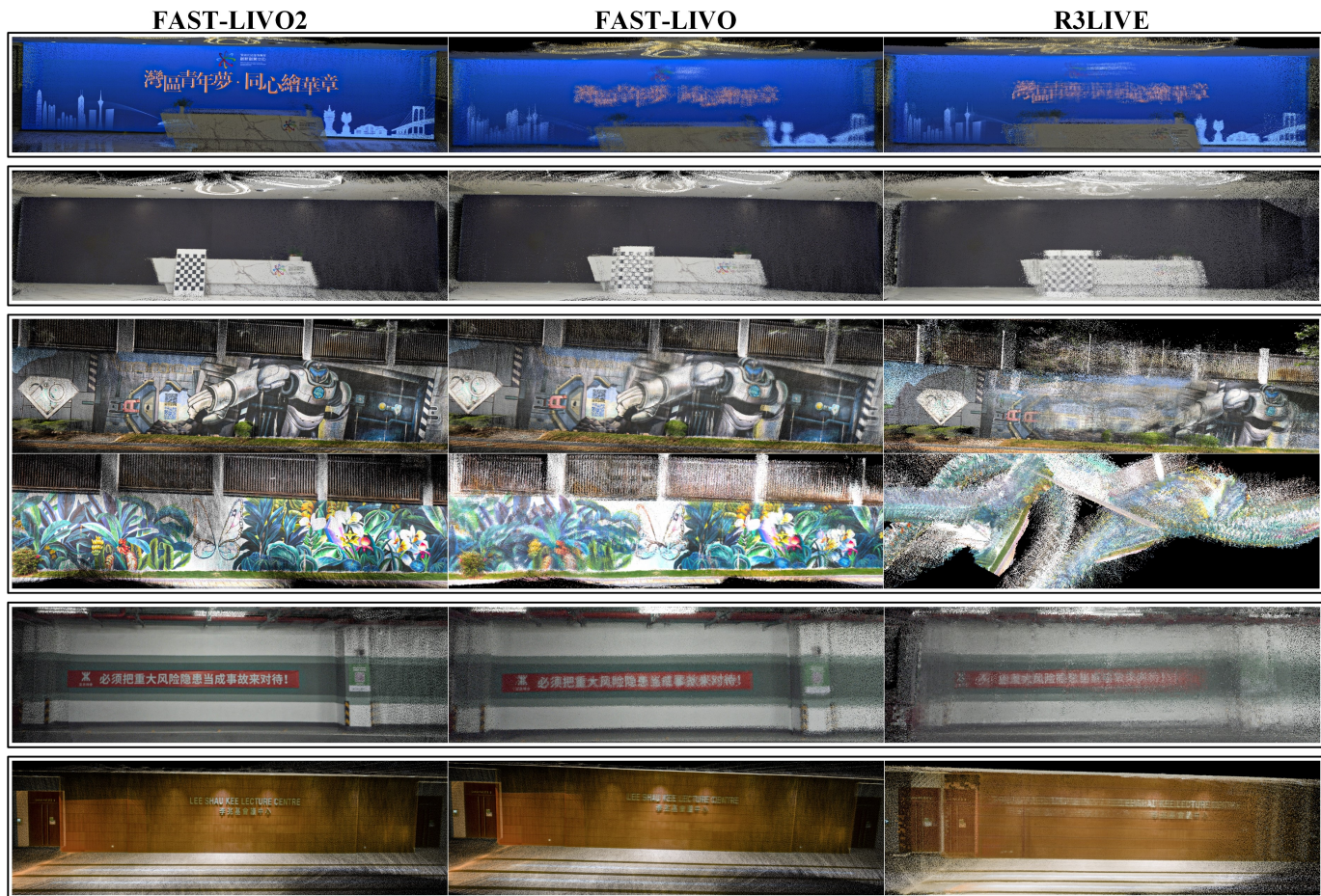
Fig. 10: The mapping results generated in real time in LiDAR degenerated scenes. The point clouds from top to bottom correspond to “Bright Screen Wall”, “Black Screen Wall”, “HIT Graffiti Wall” (the third and fourth rows), “Banner Wall”, “HKU Lecture Center”, respectively, showing the comparison of colored point cloud constructed FAST-LIVO2, FAST-LIVO or R3LIVE (see more details on YouTube: youtu.be/aSAwVqR22mo ).
