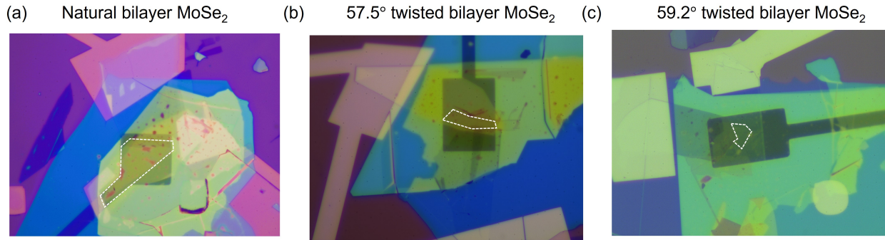
Extended Data Fig. 1: Images of samples in the main text. (a-c) Optical microscopy picture of the natural bilayer MoSe 2 (a), 57.5° twisted bilayer (b) and 59.2° bilayer (c). The white dashed line shows the twisted bilayer region. The scale bar is 10 \mu\text{m} .
