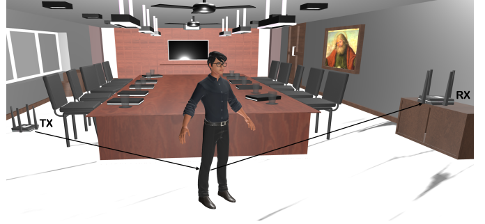
Fig. 1: Schematic diagram of WiFi signal propagation to the human body.
