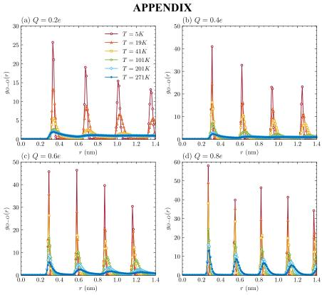
**PS. 1.** Radius distribution functions of two oxygen atoms,  $g_{O-O}(r)$ , at various temperatures under different Q values. The  $g_{O-O}(r)$  is defined by  $g_{O-O}(r) = \frac{1}{\bar{\rho}} \frac{\langle n(r) \rangle}{\Delta r}$ , where  $\langle n(r) \rangle$  is the ensemble average number of oxygen atoms in the interval  $[r, r + \Delta r]$  and  $\bar{\rho} = \frac{N}{L}$  is the average
