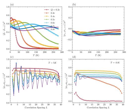
**PS. 4.** Correlations between neighbouring water molecules, including the correlations of (a) dipole vector  $\vec{\mu}_i$  and of (b) normal component  $\mu_{\perp}$ . (c) Dependence of correlation of  $\mu_{\parallel}$  on two water molecules with the spacing L at fixed temperatures of 5 K and 41 K. L represents the difference between indices of two molecules.
