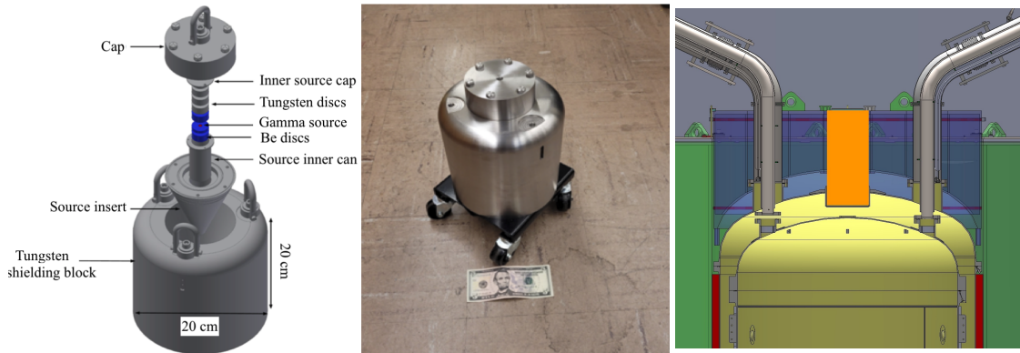
Figure 20: Left: CAD drawing for the YBe photo-neutron source assembly. The ^{88}\text{Y} sealed source is sandwiched between ^9\text{Be} disks to generate neutrons. The tungsten shielding reduces the number of ^{88}\text{Y} \gamma -rays that can enter the detector. Middle: YBe source inside the tungsten shielding placed next to a five-dollar bill for scale. Right: Layout of the top part of the OD and water tank. The custom cut-out (orange) in the acrylic vessels (purple and green) through which the YBe source is deployed is shown.
