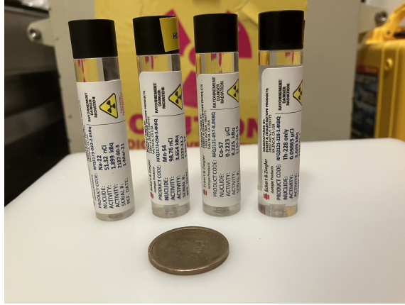
Figure 14: Picture of ^{57}\text{Co} , ^{54}\text{Mn} , ^{22}\text{Na} , and ^{228}\text{Th} \gamma -ray sources that are deployed in LZ for high energy ER calibrations.
