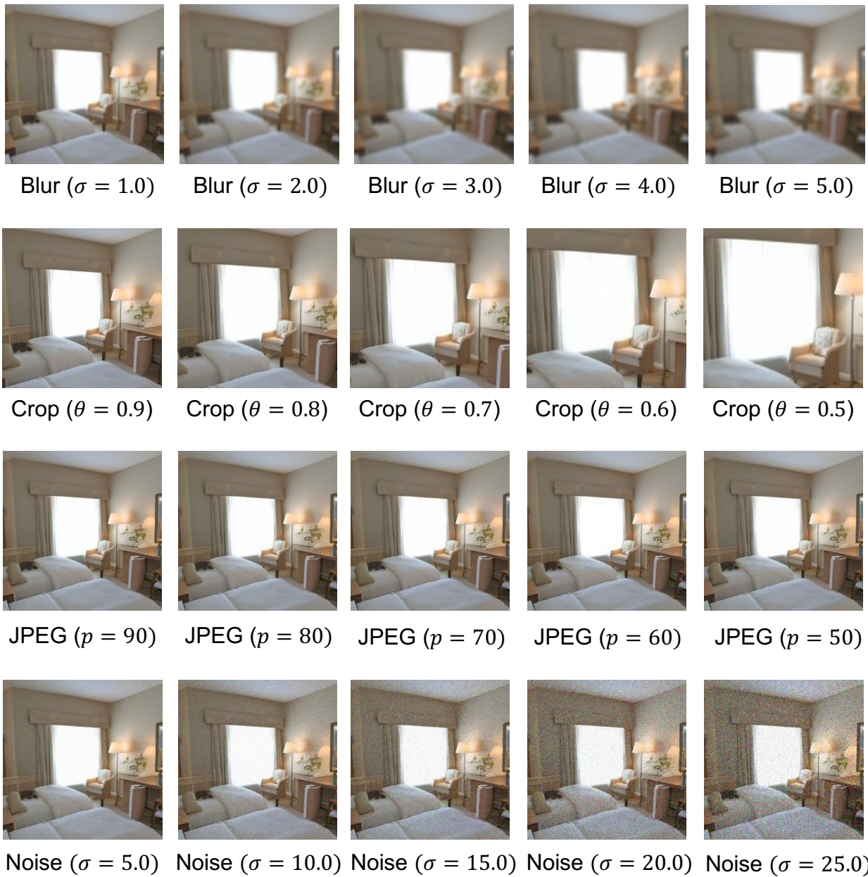
Fig. 9: Visualization of different perturbations, including Gaussian noise, Gaussian blur, cropping, and JPEG compression.
