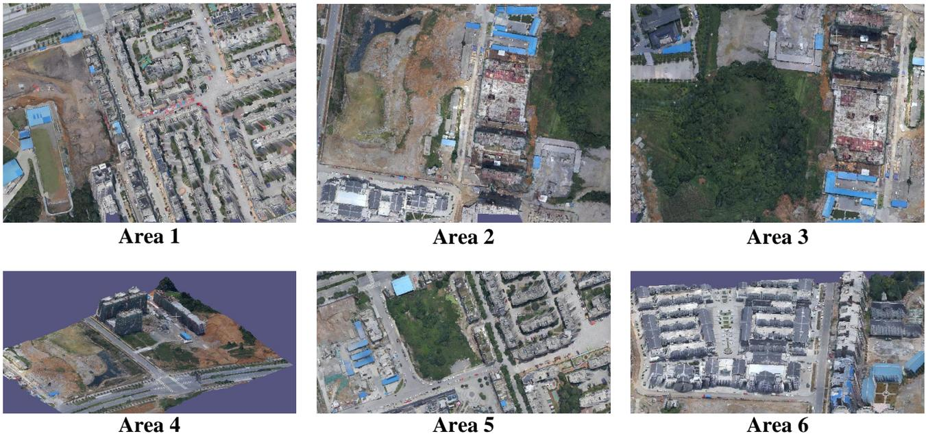
Fig. 9. Local visualization results of point cloud fusion of the proposed SDL-MVS on the WHU dataset. The point cloud results are obtained by the fusion of multi-view depth maps. We selected areas with dense buildings and areas where buildings and vegetation coexist for visualization.
