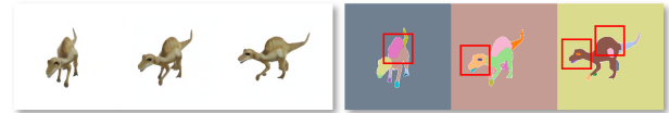
Figure 2: 2D segmentation masks without correspondence and with multi-view inconsistency (highlighted with red boxes). Left: multiview images. Right: 2D segmentation masks from SAM [Kirillov et al. 2023]; different colors indicate different parts, and there is no correspondence between masks across views.
