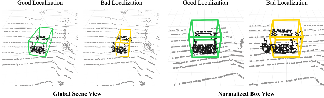
Figure 2: Example Car objects converted into normalized box view (NBV). Foreground/background points are marked in black/gray, respectively for better visualization. Foreground LiDAR points distributing tightly within a [-1, 1]^3 NBV cube is a domain-consistent sign for good localization.
