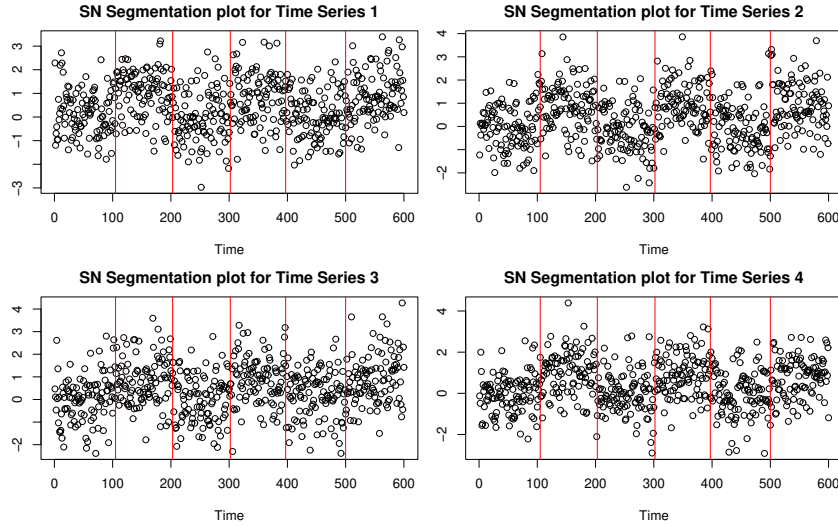
Figure 4: An example of estimating changes in high-dimensional mean for model (HD). The detected change-point locations are indicated by a red vertical line for the first 4 time series.
