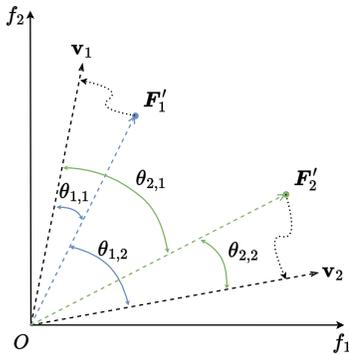
**Figure 1: Illustration of reference vector guided selection in RVEA. The population is partitioned into subpopulations by associating each with a reference vector, according to the angle-penalized distance (APD) metric.**
