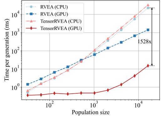
**Figure 3: Performance comparison on CPU and GPU platforms when scaling the population size on DTLZ1 problem. Results highlight the significant speedup achieved by using GPU over CPU, with TensorRVEA on GPU showing a remarkable 1528× speedup at the largest population size examined.**
