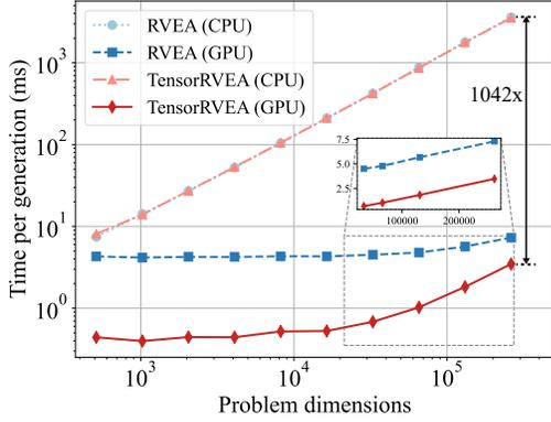
**Figure 4: Performance comparison on CPU and GPU platforms when scaling the problem dimension on DTLZ1 problem. Results highlight the significant speedup achieved by using GPU over CPU, with TensorRVEA on GPU showing a remarkable 1042× speedup at the largest problem dimension examined.**
