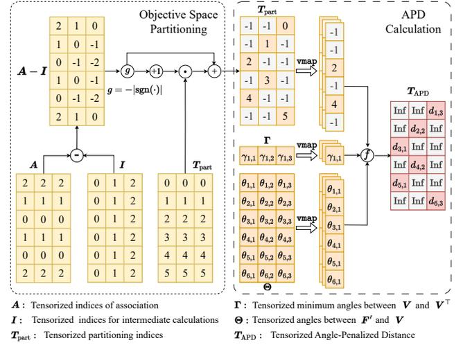
**Figure 2: Example of objective space partitioning and APD calculation for  $n = 6, r = 3$ . Left: objective space partitioning. Right: APD calculation.**
