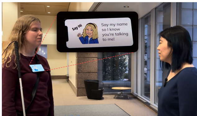
Figure 6: Pictorial Display implementation. The BLV user's Pictorial Display , worn high on their chest, reminds the sighted helper to begin by explicitly mentioning the BLV user's name. Appendix B shows all possible pictorial messages.
