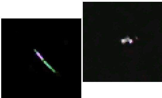
FIGURE 1. Particle detection by a smartphone. The images are transferred to a supercomputer in order to be analyzed for particle identification, usually by Machine Learning techniques.
