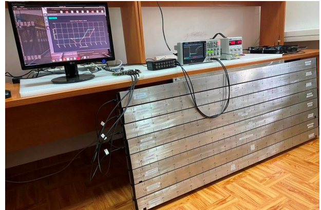
FIGURE 3. Real photo of the MCORD section during test measurements.
