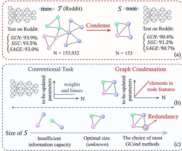
**Figure 1: The compression capability and limitations of current GCond.** (a) GCond adeptly compresses the dataset to just 0.1% of its initial size without compromising the accuracy benchmarks. (b) Contrary to traditional graph learning, GCond’s parameters scale with node count. (c) To avoid insufficient information capacity, GCond typically introduces node redundancy.
