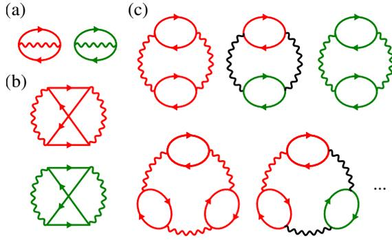
FIG. 1. The Feynman diagrams used in the calculation of the eh plasma energy. Red solid line: electron; green solid line: hole; red wavy line: Coulomb interaction between holes; green wavy line: Coulomb interaction between electrons; black wavy line: interlayer Coulomb interaction. (a) The Fock energy. (b) The second order exchange correlation energy  $E_2^{(b)}$ . (c) The RPA correlation energy  $E_{\text{corr}}$ , which includes all ring diagrams of second or higher orders.
