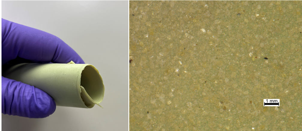
Fig. 6. Left: Polyimide aerogel scattering filter prepared as a 1mm thick film with diamond scattering particles of three size ranges, 3–6 \mu\text{m} , 10–20 \mu\text{m} , and 40–60 \mu\text{m} (run 32 as described in Supplement 1). Right: Optical microscope image of the same filter.
