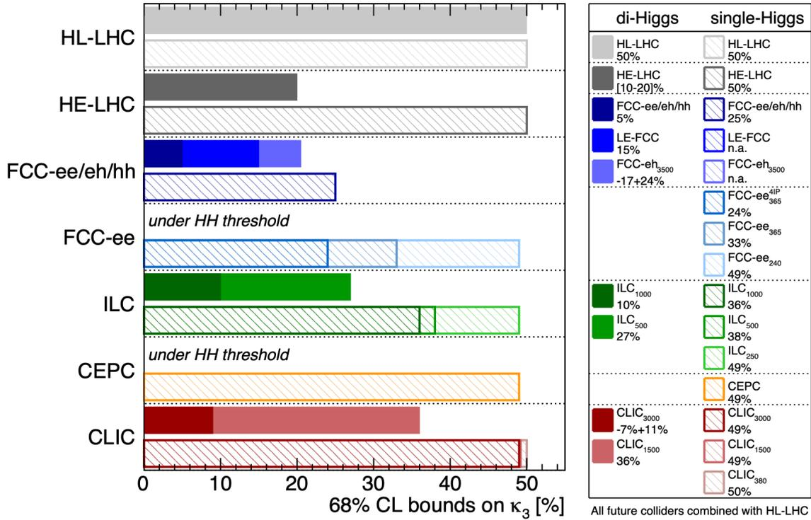
Figure 1: Sensitivity at 68% probability on the Higgs self-coupling parameter  $\lambda_{hhh}$  at the various future colliders. All the numbers reported correspond to a simplified combination of the considered collider with HL-LHC, which is approximated by a 50% constraint. For each future collider, the result from the single-Higgs from a global fit, and double-Higgs are shown separately; from the Physics Briefing Book [6] for ESUPP 2020.
